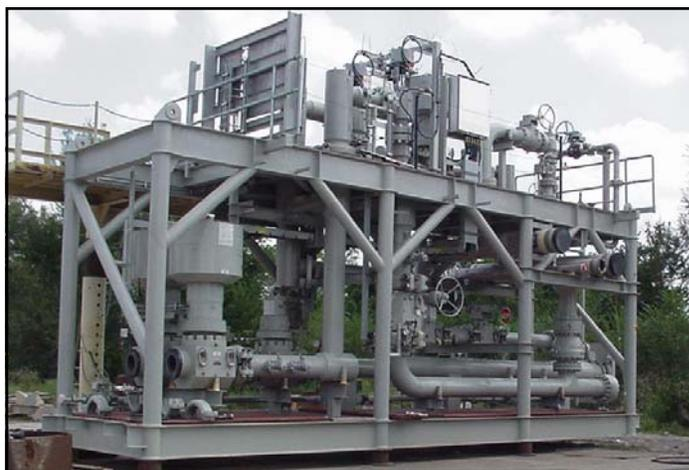
**Skid piping for flow launcher-receiver.**
